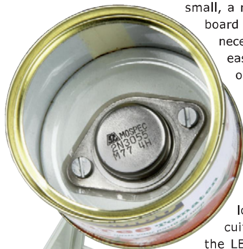
Figure 3. The mounting of the 2N3055 on the bottom of the tin. The transistor still needs to be covered with sealant to make everything waterproof.
